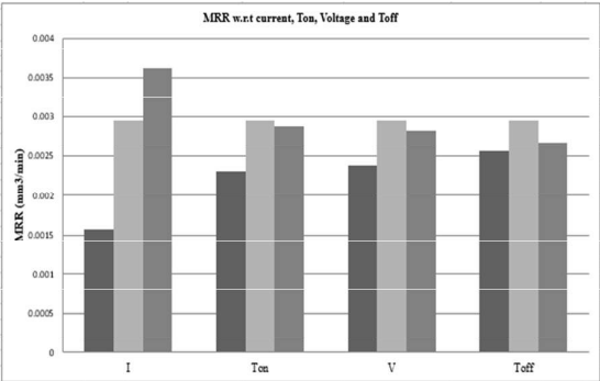
Figure 3. Variation of MRR with I, Ton, V and Toff for Cryogenic treated Copper electrodes
